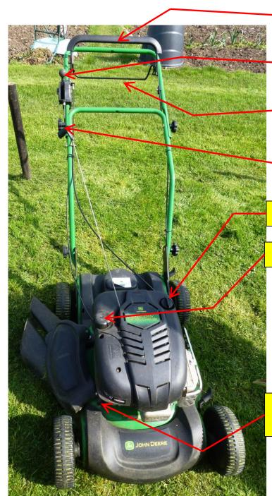
Blade Control & Engine Cut-Out Lever
